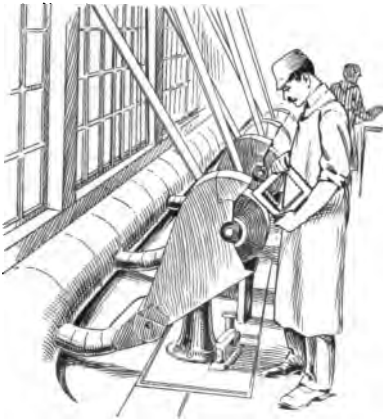
Dust exhausts on grinding wheels protect lungs of the workmen.
